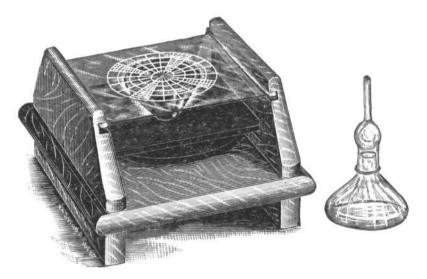
The "Wolffhüggle" device which is still so commonly employed, has the disadvantage of not firmly fixing the "Petri" dish in place, so that there is no small danger of counting the same colonies more than once. Nor is it possible to make use of a "Miquel" flask as a substitute for the "Petri" dish, if the "Wolffhuggle" counter is to be employed.
